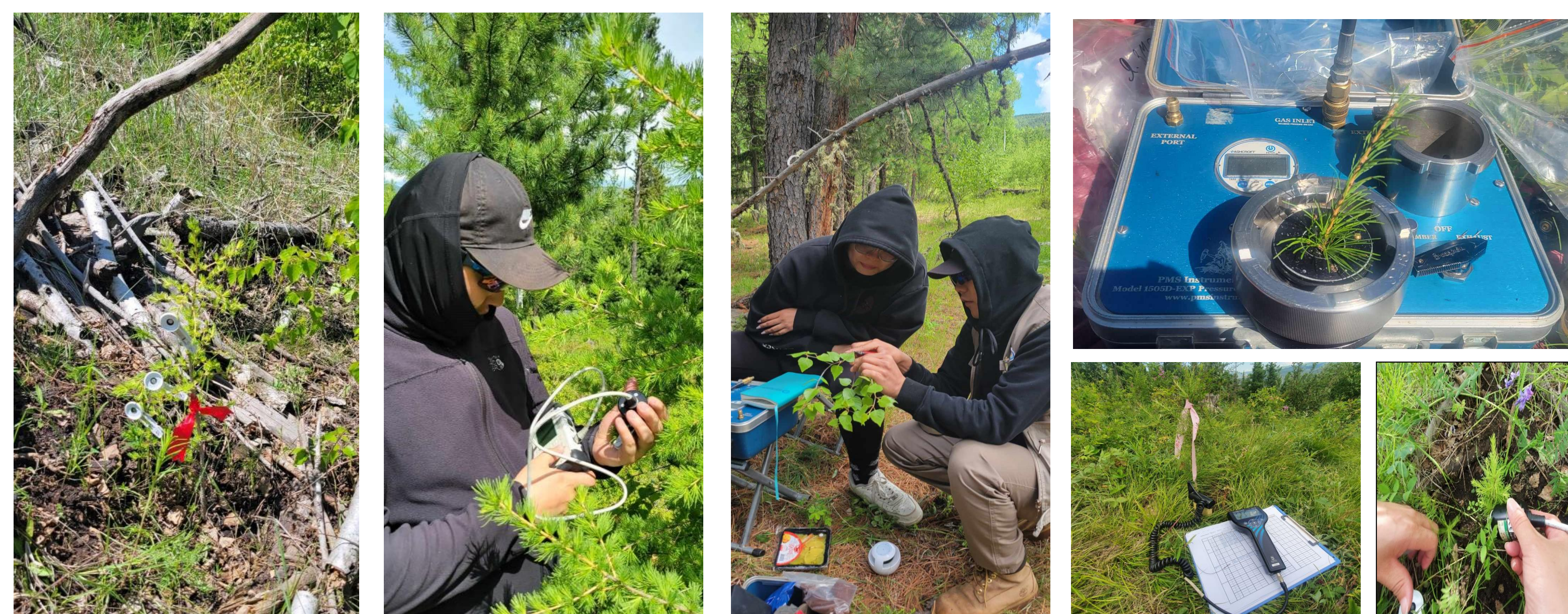
Picture 1. Measurements of chlorophyll fluorescence, water potential and soil moisture content of sample sites and sample trees
