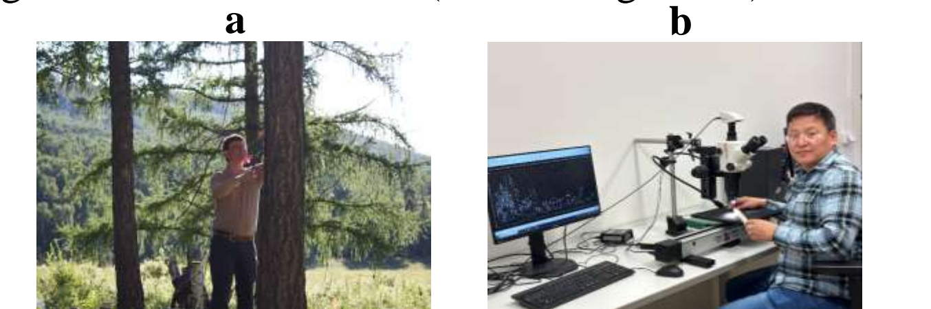
Figure 14. a) Taking core, b) measuring the core on the lintab instrument.
