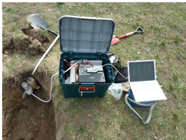
**Fig. 5** The observation system of ground temperatures, which includes a 10 m long thermistors string, a Campbell Scientific data-logger, and a laptop
