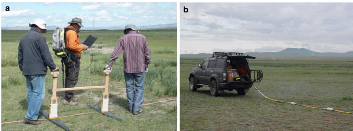
**Fig. 4** The GPR investigation with 100 MHz shielded board-shaped antenna across a 68 m long transect near the borehole (a) and 100 MHz RTA across the continuous 2.4 km, east-to-west transect (b)
