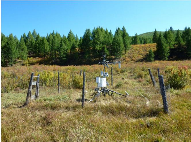
**Fig. 2.** A full view of an automatic weather station deployed at Davaat, in the continuous permafrost regions of Mongolia. The continuous observation data of ground surface temperature obtained from infrared temperature sensor were used in this study to validate the annual surface freezing/thawing index based on calculating monthly surface temperature data.
