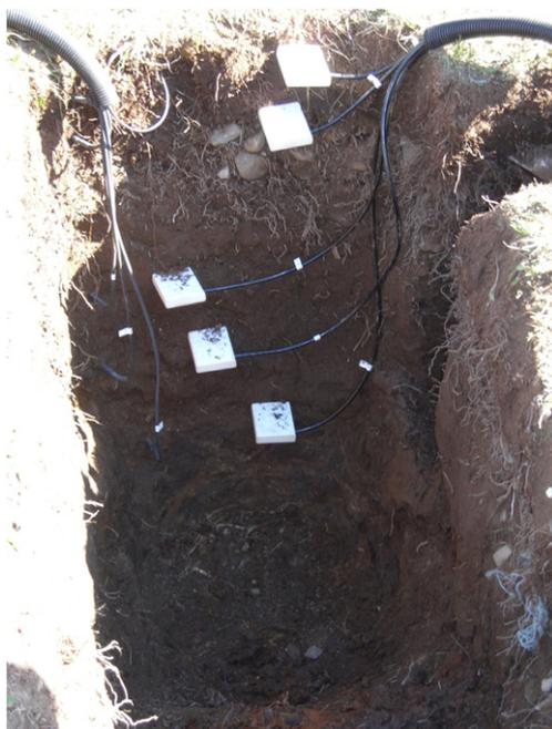
**Fig. 3.** The thermistors (PT-100) were installed in the excavated soil profile at the depth of 5 cm, 15 cm, 40 cm, 50 cm, and 65 cm respectively from the ground surface. The daily observation data from the depth of 5 cm were used to validate the annual surface freezing/thawing index based on calculating monthly surface temperature data.
