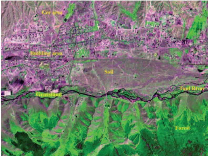
Figure 1. SPOT XS image of the selected part of Ulaanbaatar (Red=band2, Green=band3, Blue=band1). The size of the displayed area is about 13.2 \text{ km} \times 9.8 \text{ km} .
